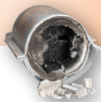
Melted Brick Engine operating too hot.
