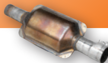
Burned Converter Exhaust temperature too hot.
