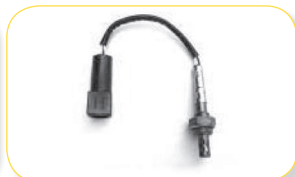
11015 1983-86 Ford, Lincoln, Mercury 3-wire w/ connector
