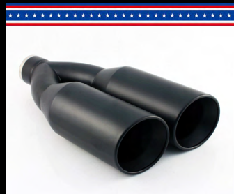
DT-30538DSBK BLACK POWDER COATED 5" DUAL SIDEWAYS DOUBLE WALL ROLLED EDGE
