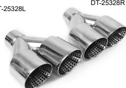
DT-25328CL, DT-25328CR DUAL POLISHED EXHAUST TIP DRIVER & PASSENGER SIDE ID 02.50" OL 09.50" OD 08.25" (4" x 2) PK 5
